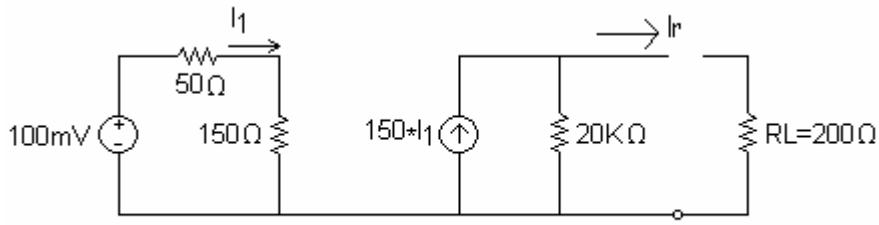
Por Ohm:  $I_1 = \frac{100mV}{200\Omega} = 0.5mA$
