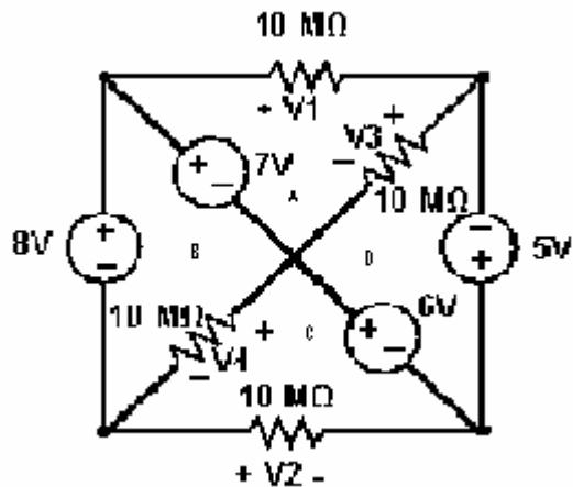
$$\text{Malla B: } 8V - 7V - V_4 = 0 \rightarrow V_4 = 1V$$
