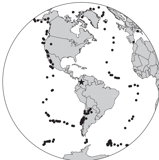
Fig. 2. Location of seismic events used for the P-wave velocity analysis. Selected earthquakes occurred during 2008, 2009 and 2010, have a magnitude of 5.5 (MI or Mw) or greater, and are located at epicentral distances between 30 and 90° from Bogotá, Colombia (star).
