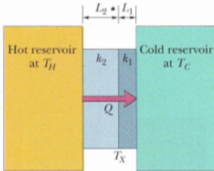
$$P_{\text{cond}} = \frac{k_2 A (T_H - T_X)}{L_2} = \frac{k_1 A (T_X - T_C)}{L_1}$$
